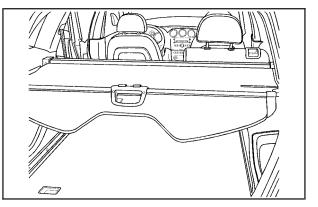
Your vehicle may have a cargo cover. It can be used to cover items in the rear of the vehicle. Pull the cover toward the rear of the vehicle and place each end in the slots provided. To install the cover, place each end of the cover in the holes behind the rear seat. To remove the cover, pull both ends toward each other.
